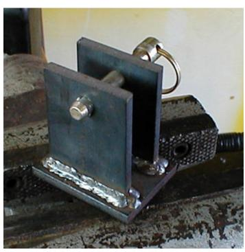
The problem was these trailers are used by a number of tow vehicles, from mowers to carryalls, and even golf carts. We came up with a fairly simple hitch to make in house. Using 1/4 X 2 flat stock, we cut pieces 2 1/2" long. Then clamping two together, drilled them with a 3/8 bit in a vise. To keep the holes aligned we used a long carriage bolt and lock the pieces in place with nuts.
